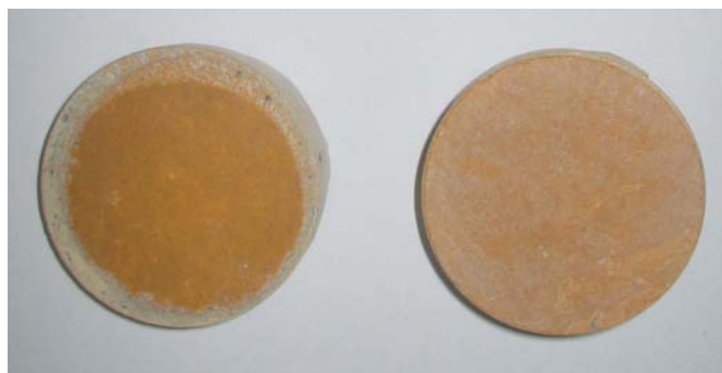
Figure 4 Core drill samples of a yellow magnesia floor from southern Germany. The yellow colour was achieved by mixing iron oxides into the MgO powder. Left: correctly colored sample; right: bleached sample.
